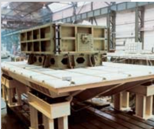
Vibrating tables with continuously adjustable magnetic vibrators ensure perfect material compaction in production and during packing
