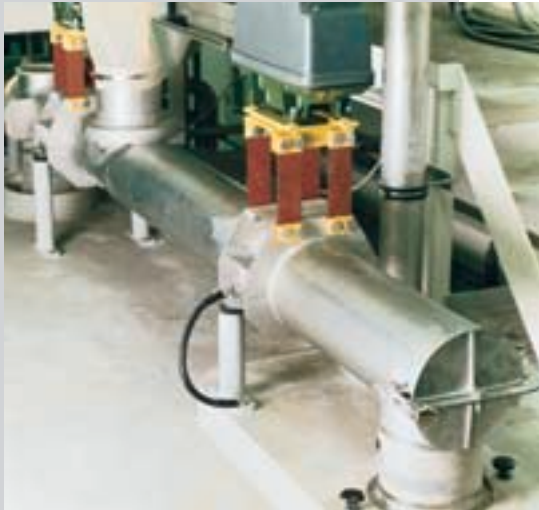
A reversible tubular conveyor distributes milk powder alternately in two directions. The 100% turnaround in the material flow is achieved by electrical switching, without complicated flap mechanisms
